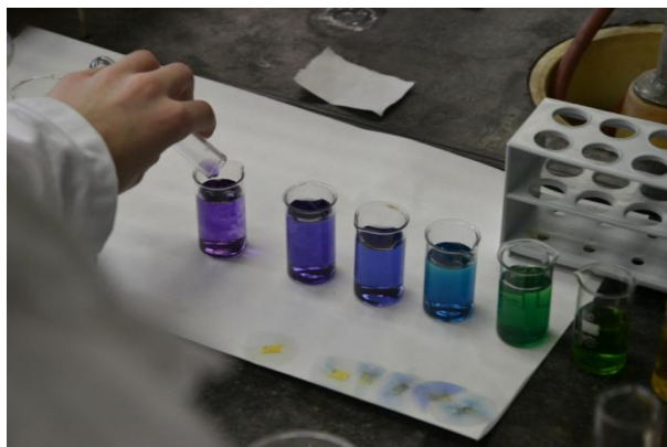
Pic. 3 Verification of pH scale with available indicators – extract of red cabbage (foto: Šponiar)
