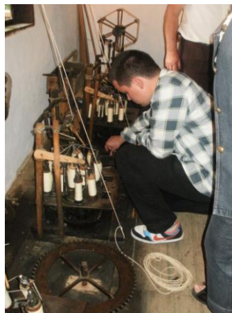
Fig.2. Knitting “gaytan” with the help of a special cog wheel mechanism called a “chark”
