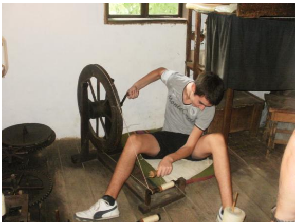
Fig.1. Winding the yarn on the spools with the help of a spinning wheel (“chekrak”)
